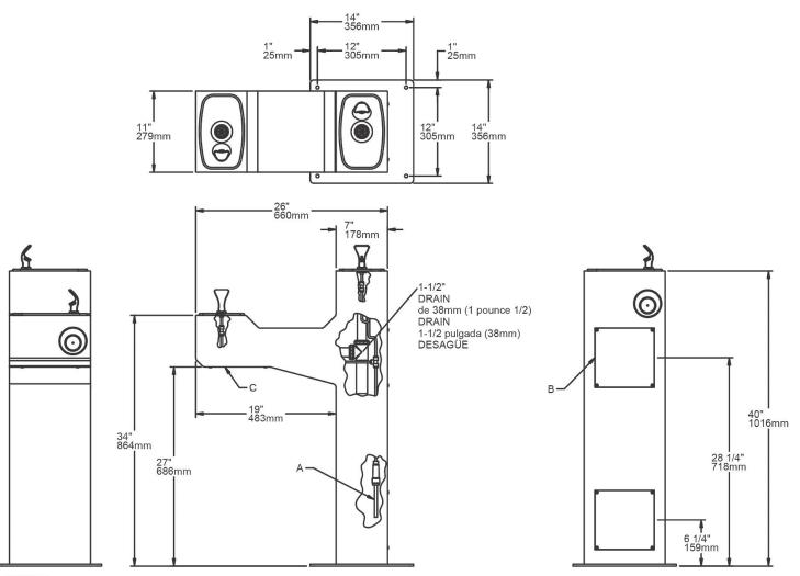
A = 3/8" (10mm) O.D. unplated copper tube connect - shut off valve by others. B = Access panel. C = Removable bottom cover.
